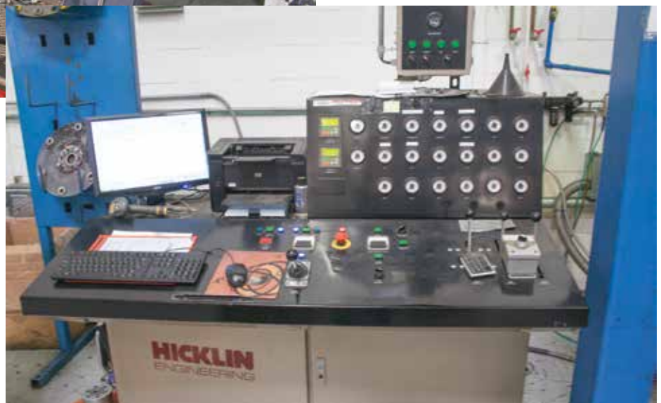
One of our Dynamometers in the process of testing an Allison transmission reman.
