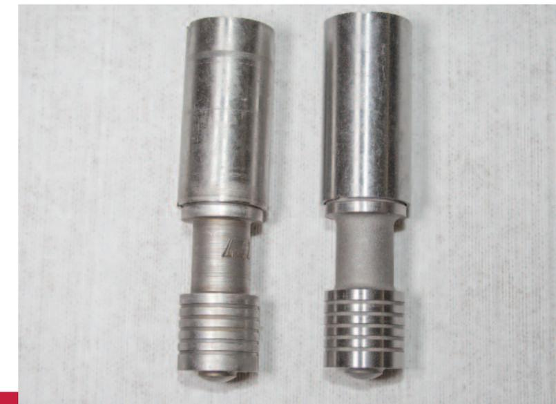
These are the valves that should have been installed with the RMC kit.
