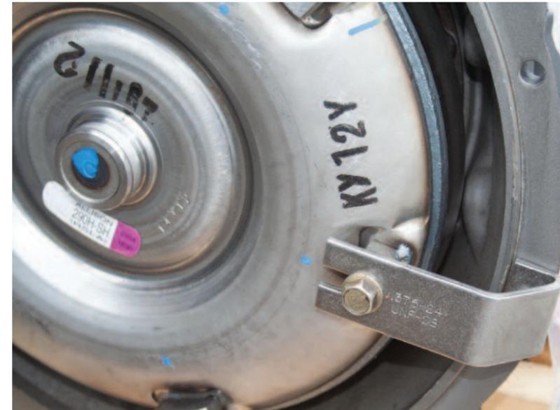
The TRC torque converter is brand-new, per Allison spec. Also note that the transport retainer is properly installed.
