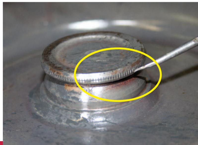
Signs of visible wear and distortion on the competitor's torque converter's knurled edges which can cause adaptation issues and premature failure.
